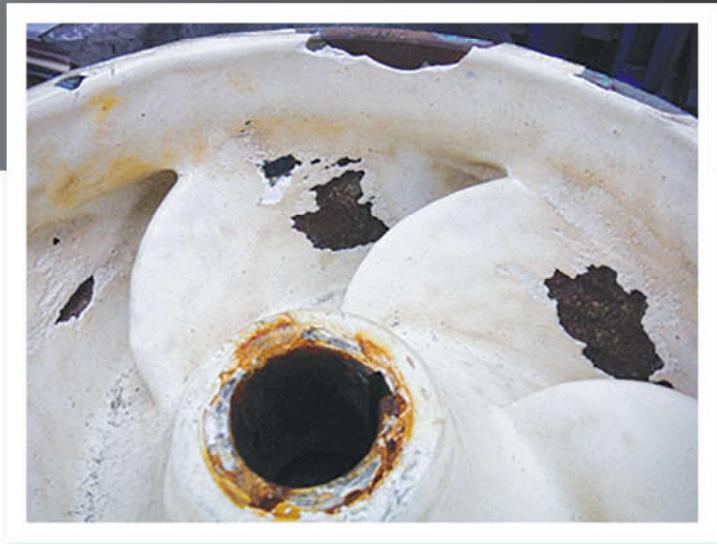
The above picture is an example of how quickly coatings fail on rotating impellers from the high fluid velocities!
